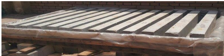
Fig. 2: Beams in group G1 placed in boxes outdoors
