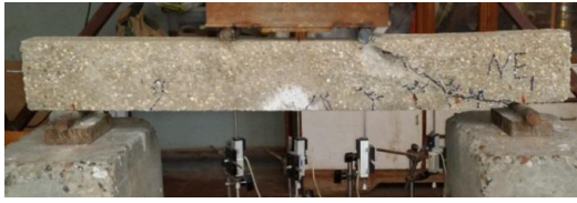
fig.23: shows failure mode of un wrapped
