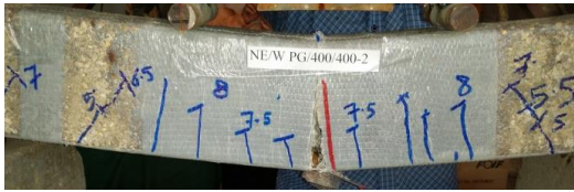
(a) Flexure failure
