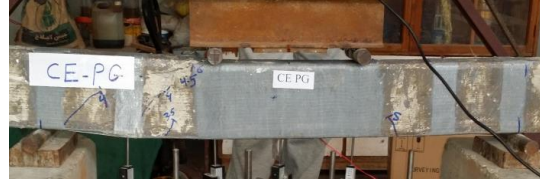
(b) shear failure
